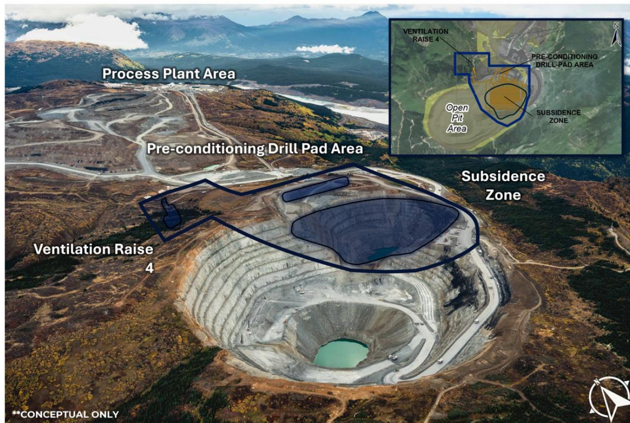
Figure 1-15: Conceptual Representation of Block Cave Components and Associated Project Footprint
